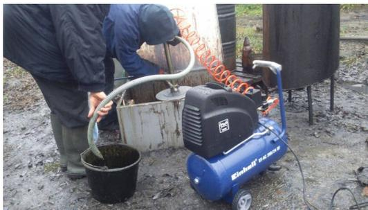
Mobile pneumatic skimming system for floating phase
